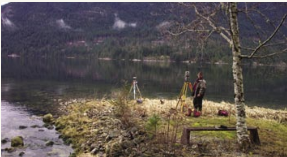
Crown land survey in Narrows Inlet: Dan Fennings at the total station (similar to a theodolite) with GPS set up for additional control
