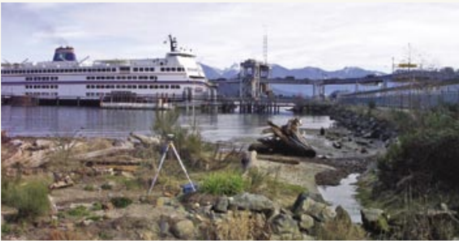
GPS survey control for foreshore lease survey at the Langdale ferry terminal
