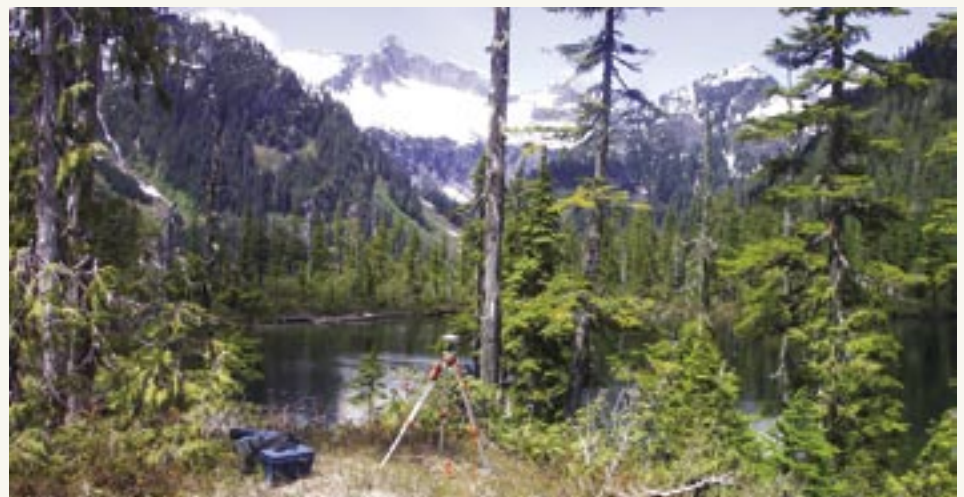
GPS survey control in sub-alpine (helicopter access only) for topographical survey work on an independent power project
